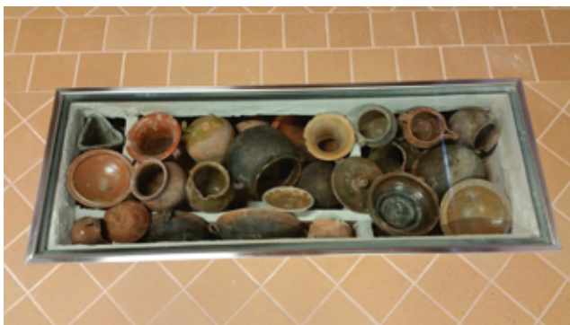
Fig. 3. Vases used as fillers in the vaults of Vic's cathedral, 14 th century (image courtesy of Judit Molera).
